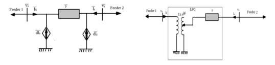
Fig IV (c): Circuit model of loop power controller.
