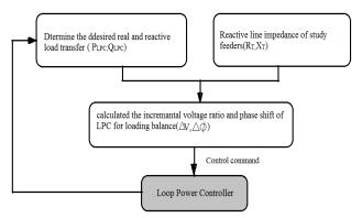
Fig IV (b): Flowchart of LPC control algorithm.
