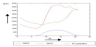
Fig V (b): Power profiles of Feeder MF65 and MU67 (with FC system).
