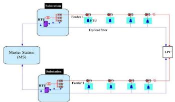
Fig IV (a): Distribution automation system with a loop power controller
