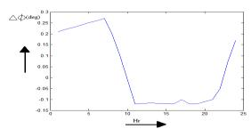
Fig V (e): phase shift for the power transfer by LPC (w/o FC system)
