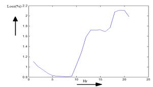
Fig V (h): Percentage of system power loss before applying LPC for loading balance (with FC system).
