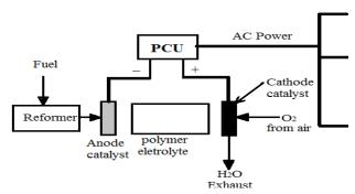
Fig III (a): Configuration of the fuel cell system
