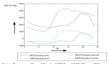
Fig V (a): Power profiles of Feeder MF65 and MU67 (w/o FC system).
