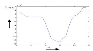
Fig V (d): voltage ratio for the power transfer by LPC (w/o FC system)
